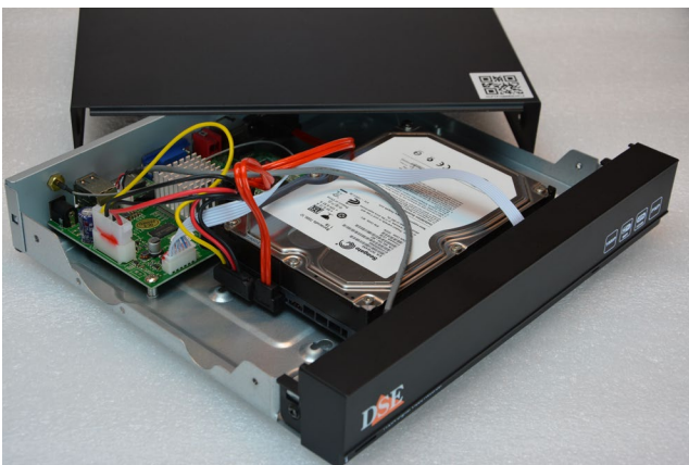
Secure the hard disk with the 4 screws provided screw from underneath the base. Then close the cover.
