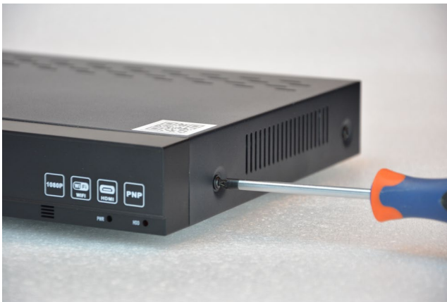
Remove the cover by unscrewing the 5 screws: 2 on each side and one on the back
